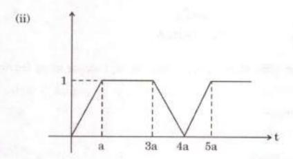
Obtain the Laplace transform of the following periodic waveforms:
