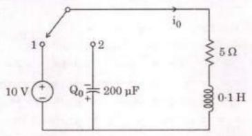
In the series RLC circuit shown in the figure, the capacitor has an initial charge  $Q_0 = 1$  mC and the switch is in position 1 long enough to establish the steady state. Find the transient current which results when the switch is moved from position 1 to 2 at t=0.
