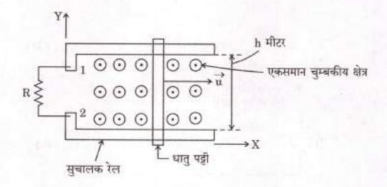
A metal bar slides over a pair of conducting rails in a uniform magnetic field  $\overrightarrow{B} = \overrightarrow{a}_z \ B_0 \ Wb/m^2$  with a constant velocity  $\overrightarrow{u}$  m/s as shown below in the figure. A resistance 'R'  $\Omega$  is connected between terminals 1 and 2. Prove that this system upholds the principle of conservation of energy. Neglect the electrical resistance of the metal bar and the pair of conducting rails, and the mechanical friction of this ideal system.
