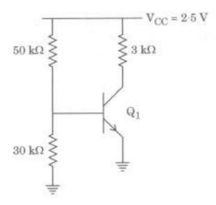
For the circuit shown below, early voltage  $V_A = \infty$  and  $\beta = 100$ . Find the reverse saturation current if:
