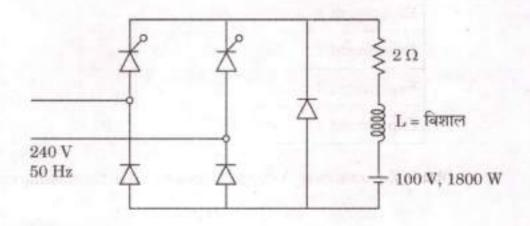
A half-controlled converter fed from 240 V, 50 Hz single-phase ac source is feeding 1800 W power to a 100 V battery as shown in the figure below. The battery is connected in series with a large inductance and a resistance of 2  $\Omega$ . The inductance is large enough to make the load current flat and continuous.
