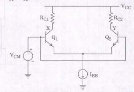
Consider the figure of differential pair given below. Neglecting the early effect, determine the change in  $V_X$ ,  $V_Y$ ,  $V_X$  –  $V_Y$
