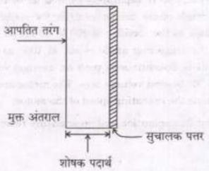
An absorber material of relative permeability and relative permittivity of  $\varepsilon_{\rm r} = \mu_{\rm r} = 6$  – j6 is coated on a perfectly conducting sheet and this combination is placed in free space as shown in the figure given below. A 500 MHz wave is incident on it normally from free space. Calculate the thickness of the absorber required to attenuate the reflected wave by 30 dB.
